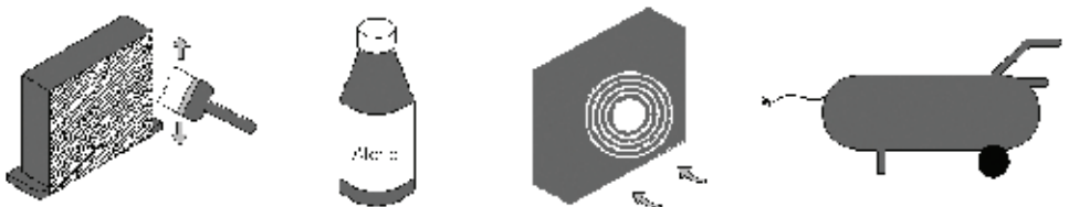
Figure 6 Cleaning of the Condenser
